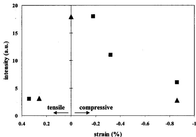
FIG. 5. Peak PL intensity vs strain at 10 K. (Squares) 9 nm QWs. (Triangles) 3 nm QWs. An unstrained QW is three times as intense as its highly strained counterpart.
