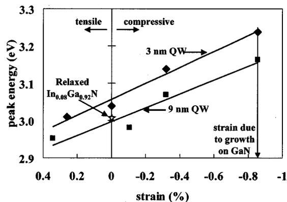
FIG. 3. PL peak energy vs strain for  $\text{In}_{0.08}\text{Ga}_{0.92}\text{N}$  QWs. (Diamonds) 3 nm QWs. (Squares) 9 nm QWs. The star indicates the band gap for fully relaxed  $\text{In}_{0.08}\text{Ga}_{0.92}\text{N}$ . The strain equivalent of growth on GaN occurs at 0.86% compressive stress.
