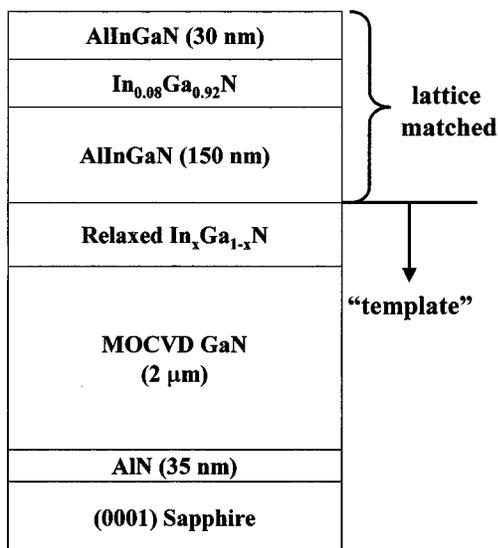
FIG. 1. Cross section of test structure grown.  $\text{In}_{0.08}\text{Ga}_{0.92}\text{N}$  QW and AlInGaN cladding are pseudomorphic to the relaxed InGaN layer. Strain is varied by changing  $x$ .
