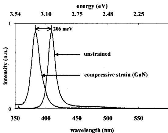
FIG. 2. Room temperature PL of 3 nm QWs under compressive and zero strain. Peak energy shifts by 206 meV going from compressive to zero strain.
