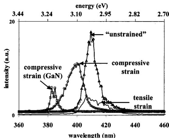
FIG. 4. 10 K PL for 9 nm  $\text{In}_{0.08}\text{Ga}_{0.92}\text{N}$  QWs subjected to varying amounts of lattice-mismatch induced strain.
